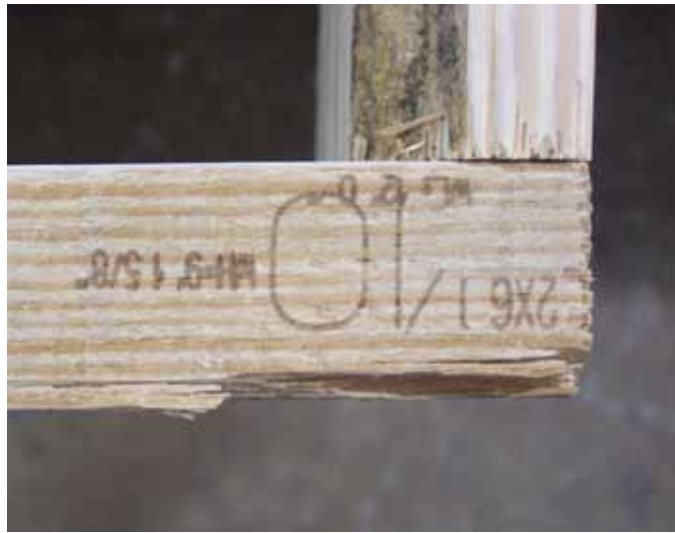
New wall panel laser machine marks wall panel dimension details in the wood.
