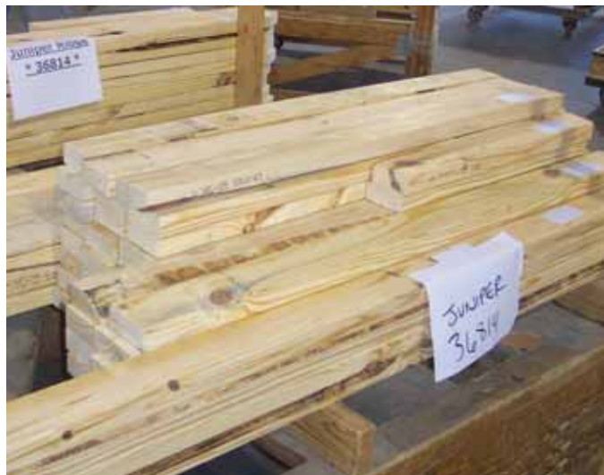
Webs are neatly stacked on a cart according to their placement in the truss and labeled with the job title and number.
