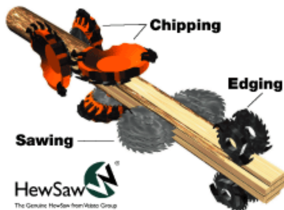
FIGURE 2. CHIP 'N SAW DIAGRAM COURTESY OF HEWSAW MACHINES INC. CLICK ON IMAGE FOR LARGER VIEW
