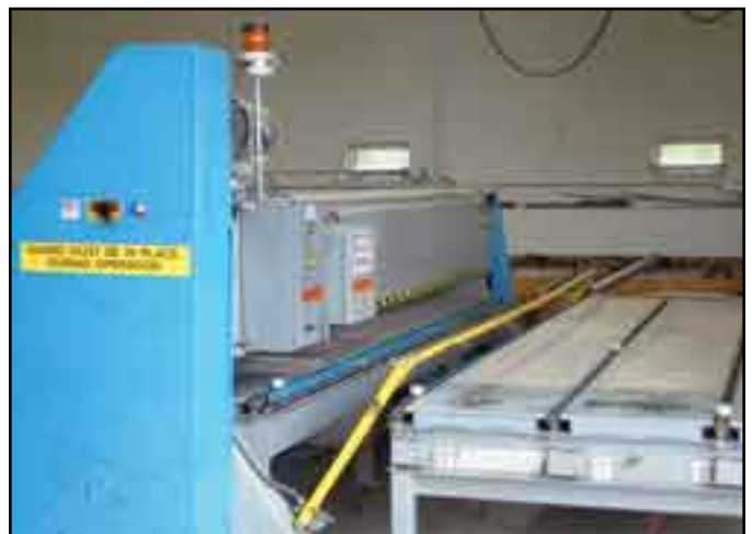
Roller gantry head on the plastic topped table with trip lever safety brake arm.
