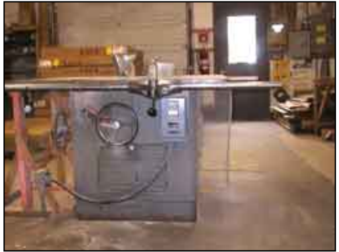
View of the retrofitted guarding on the table saw. Note the blade guards and anti-kickback guards are in place as required.
