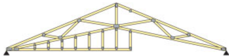
A Scissor Truss with Non-Structural Filler
