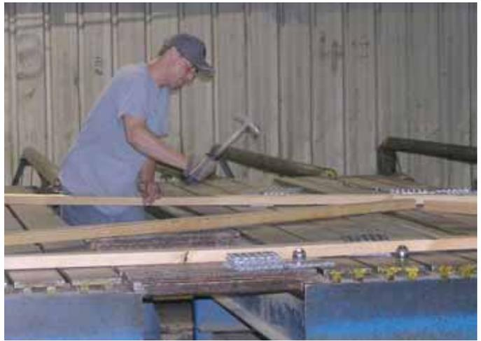
Metal connector plates are hammered into place on a wood truss.
