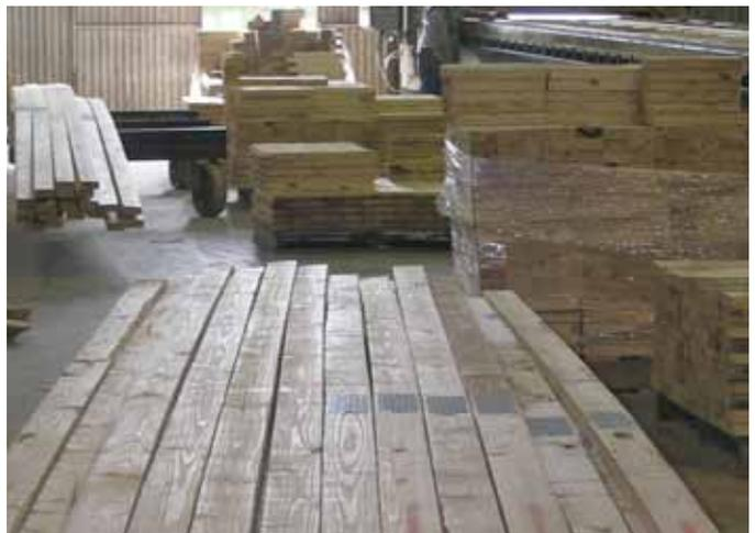
Wood floor truss chords are fastened together with metal connector plates and stacked before they are transported to the floor truss set-up tables. The floor and roof truss assembly stations are housed in one large building.
