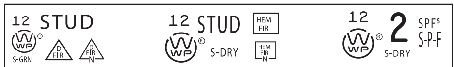
Figure 1. Lumber produced from a mix of U.S. and Canadian logs must carry a grade stamp showing species group designations.
