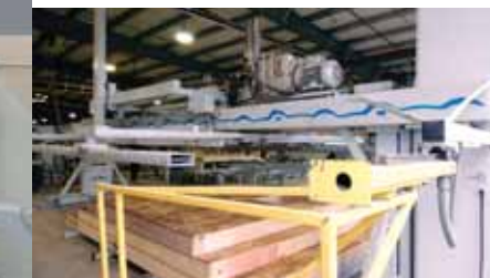
Automated Panel Stacker
