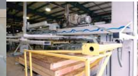
Automated Panel Stacker
