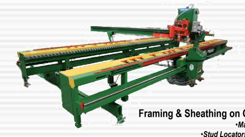
•Manual Auto Stops •Stud Locators 16" and 24" o/c Manual Frame Nailing •Quick Disconnect Air Fittings for Hand Tools Automated Sheathing Nailing Simple to Use Controls Tilt Nailing High Load Coil Capacity Infinite o/c spacing •Quick Change Tool Mounts •2x4, 2x6, and 2x8 capable Programmable for Under and Overhung Sheathing
