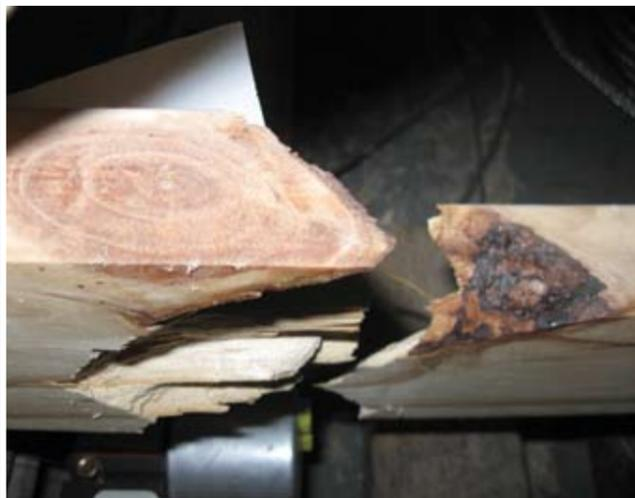
The truss fails at the spot of the knot, exposing a weakness in the lumber at that location.
