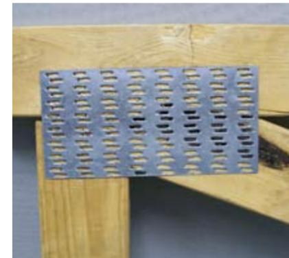
Figure 2. Pitch-pocket under plate area.
