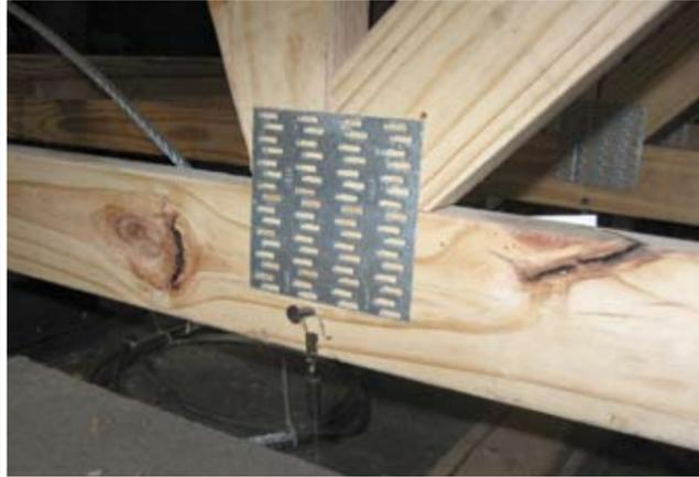
The joint of a truss in the Structural Building Components Research Institute (SCBRI) before the truss is tested. Note the knot on the edge of the bottom chord.
