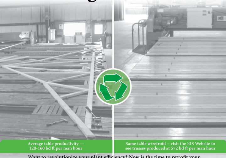
Want to revolutionize your plant efficiency? Now is the time to retrofit your assembly table with WizardPDS® drop-in ChannelS™ and eliminate ALL setup time and manual jigging. WizardPDS® drop-in ChannelS™ will retrofit with virtually any truss assembly table; new, used or existing!
