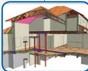
With the Section Cut View you can create a slice-through model showing the critical member elevations and relationships inside of the model.
