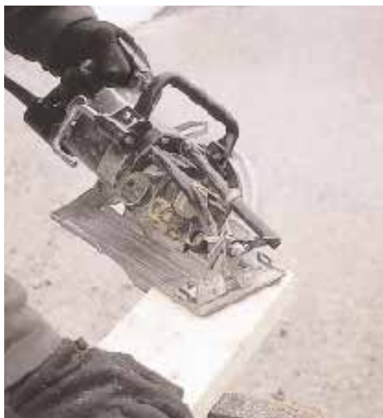
Figure 4. To make a double-cheek cut on a hip, the author lays out a plumb cut with a framing square. He marks both sides of the 1½-inch tongue on the square (above). Leaving the line visible on the board, he then cuts along the outside line with the saw set at a 45-degree bevel, moving from the top edge of the rafter towards the bottom to cut the long point (middle). Finally, he cuts in the opposite direction to cut the short point, resulting in a near-perfect double cheek cut (left).
